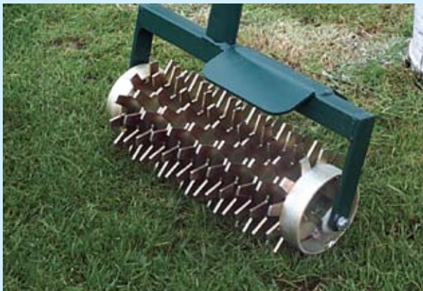
A seed slotter can create hundreds of holes for introducing new seed
