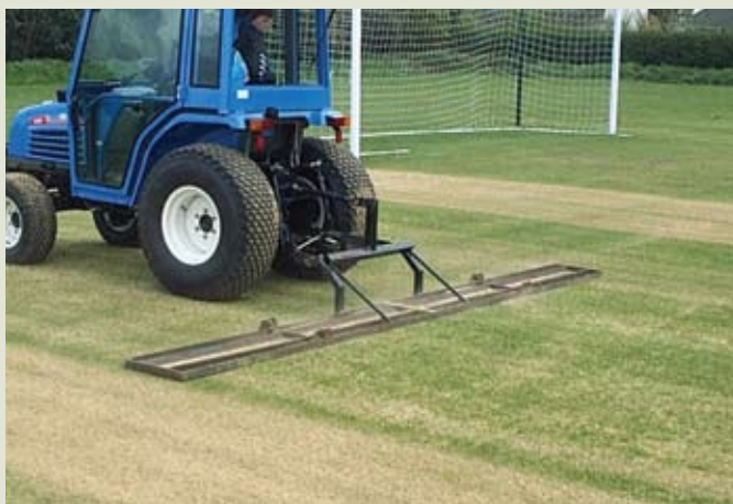
Above: A top dresser fitted with a drop brush. This is ideal for concentrated dressings.
