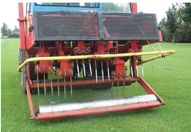
Above: A verti drain fitted with 12mm solid tines
