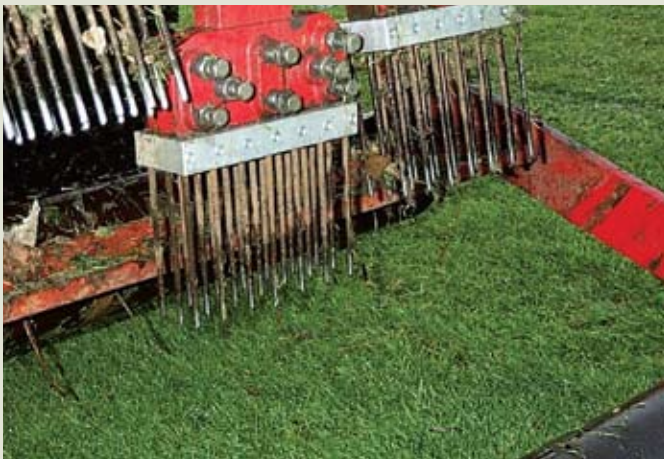
Left: A verti drain with pencil tines gives other options at renovation time
