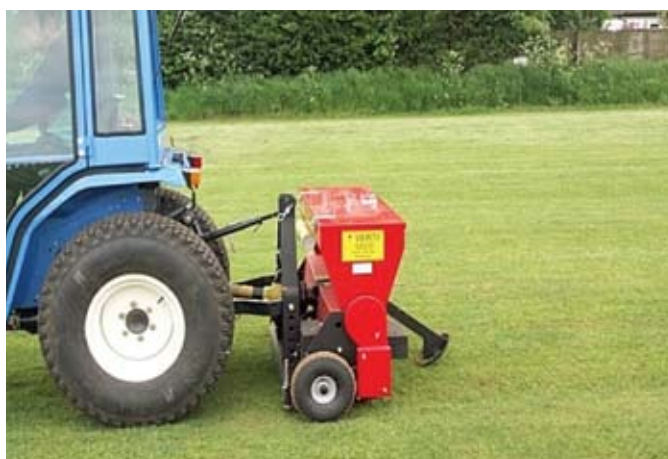
Left: The verti seeder gives very close centre drills ideal for producing a tight sward
