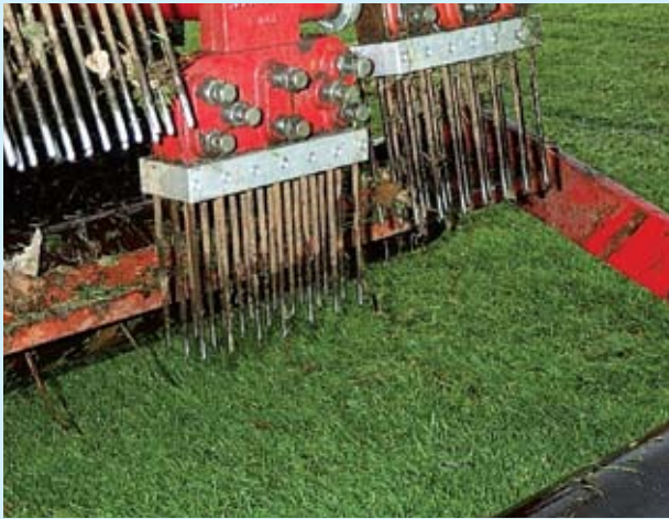
Close centred pencil tines are good for creating access for new root to develop in to
