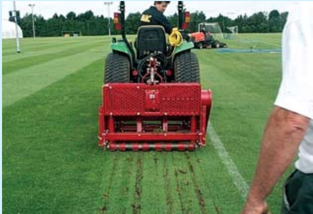
A Blec aerator cuts and slices through compact soil
