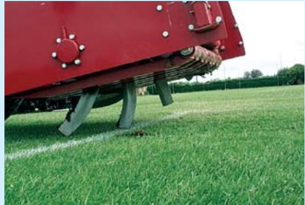
A side view showing the Blec's slicing tines
