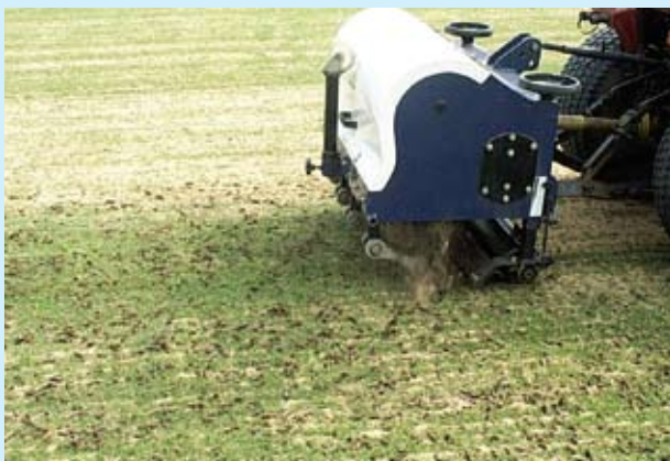
Hollow cores being punched out ready to mix with new material
